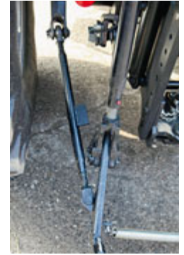
UK/Irish spec tractors come with a Dromone push-back hitch, while the ineffective stabilisers (right) can be replaced by Walterscheid options. Mudguards are scheduled for strengthening.
